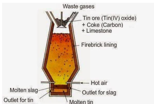
Figure 2.5: The furnace for extraction of Tin
